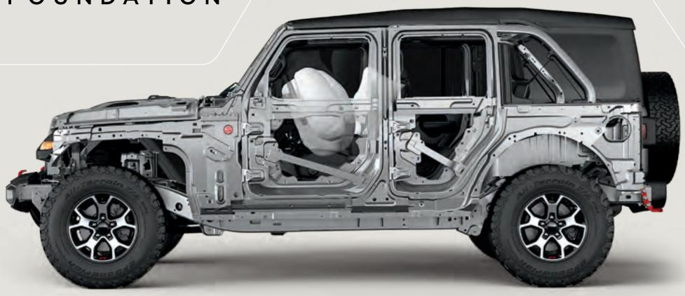
**BODY STRENGTH** The exceptionally solid safety cage consists of high-strength steel paired with lightweight aluminum, making Wrangler lighter in weight while still providing a very strong chassis. Standard.
