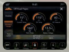
OFF-ROAD PAGES Access real-time performance data like suspension travel or keep an eye on your tilt-and-pitch. In-depth vehicle diagnostics, including wheel turn, articulation and transmission temperature, all help to provide an optimized experience. Available.
